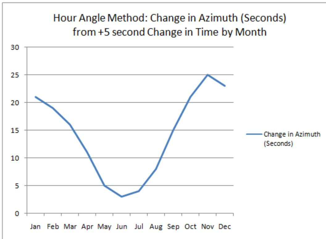
Fig.4 Hour Angle Method: Effect on Azimuth by a 5-Second Change in Time
