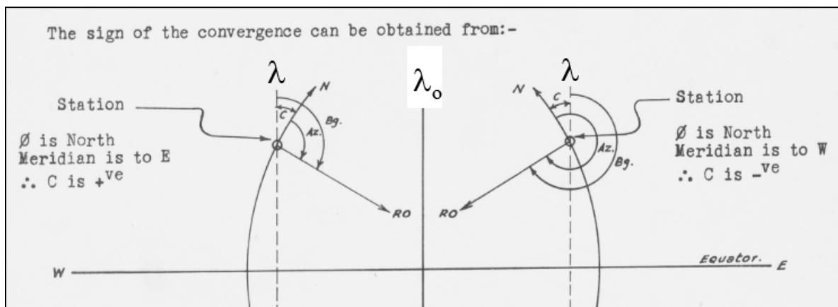
Fig.6 Grid Convergence Angle on both Sides of the Central Meridian
