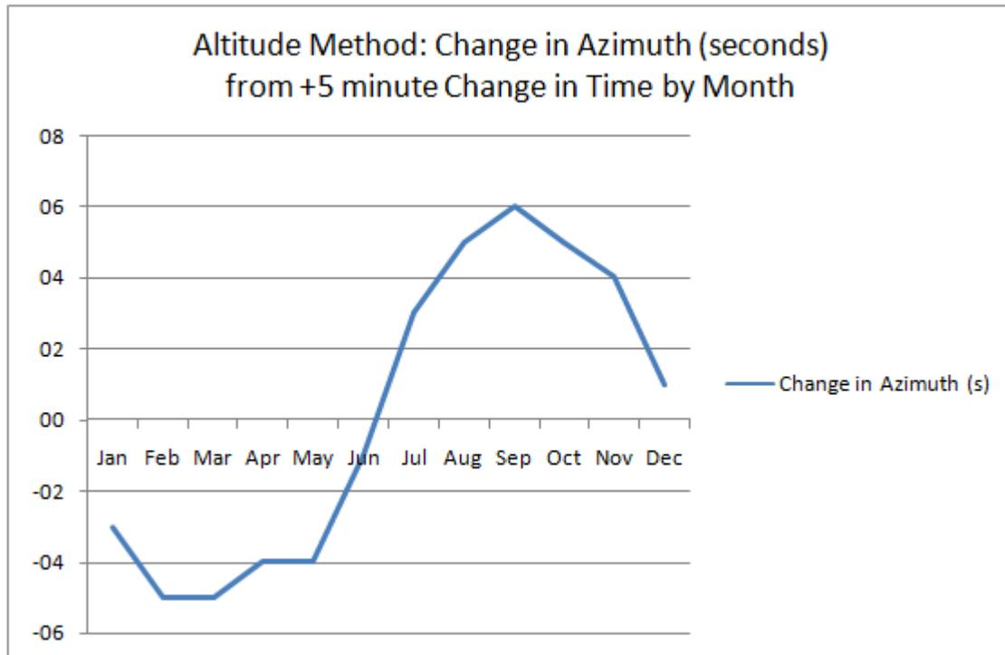
Fig.2 Altitude Method: Effect on Azimuth by 5-Minute Change in Time
